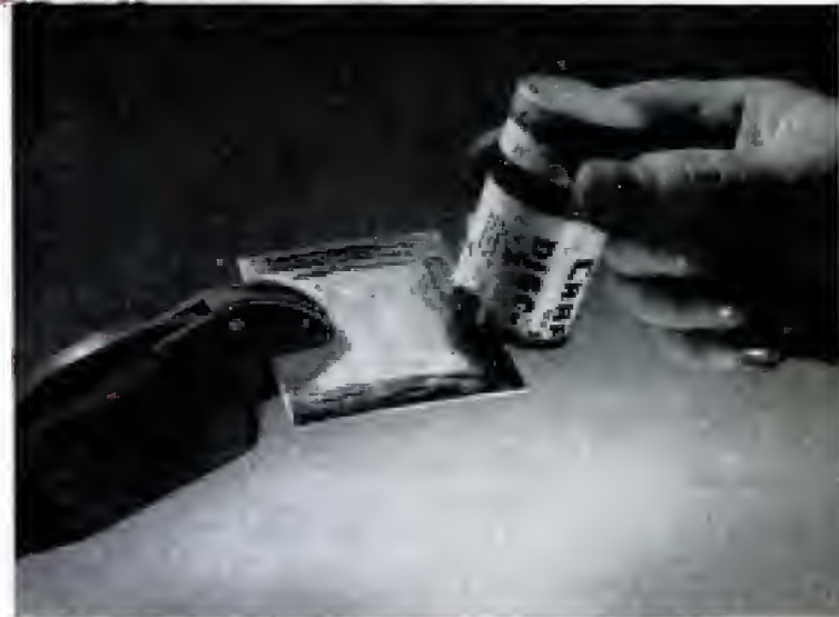
Disk cement will hold thin squares of sheet metal when stacked for jigsawing duplicate patterns. Warm the metal and apply cement to the edges as shown
